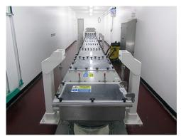
second conveyor, 24"W x 8"D x 28'-1"L, and the third conveyor at 24"W x 8"D x 64'-0"L. Adding new conveyors and modifying their existing conveyors gave them the ability to increase capacity with the addition of the two new silos. Pictured on the left, is a Slipstick Sanitary Horizontal Motion Conveyor they purchased in the 1990s and modified to extend the pan length. This conveyor going through the wall, is fed from the conveyors under the silos.
