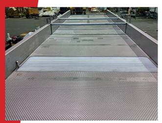
Design Requirements Product Type: Meatballs and pizza toppings Capacity: 13,000 pounds per hour Duty: 24/7 Conveyor Pan Size: 38" W x 6"D x 13.06' L
