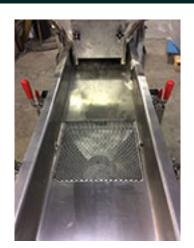
Design Requirements Product Type: Freeze-Dried Pet Treats Capacity: 2,000 Pounds Per Hour Duty: 24/7 Conveyor Pan Size: 13"W x 5"D x 5'-0" L
