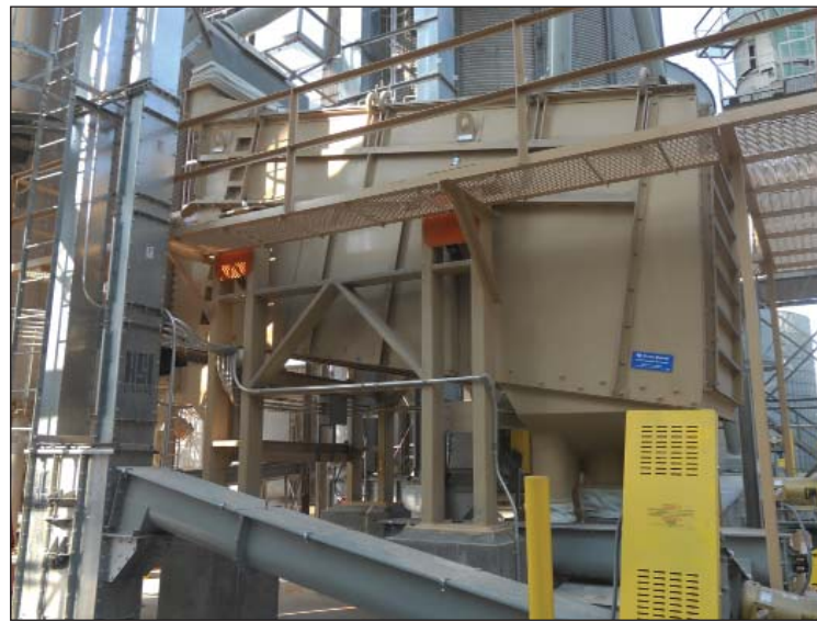
The Texas Shaker can separate dissimilar dry products at rates of 1,000 pounds per hour to 40,000 bph.
