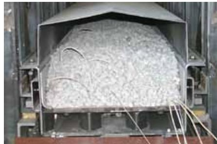
*The Slipstick can be provided in lengths of over two hundred feet equipped with a single drive unit.*
