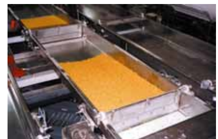
Product dams and discharge gates, actuated by downstream level sensors build product inventory and deliver on demand to packaging.
