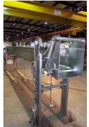
Pneumatically controlled discharge regulators prevent product surges at discharge.
