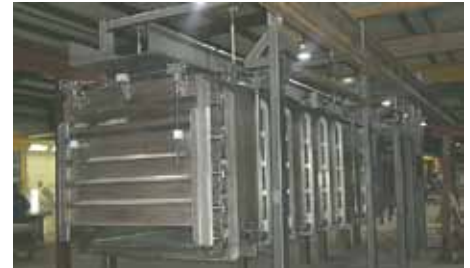
Large volumes of product are gently retained with the discharge rate controlled by an adjustable height weir.
