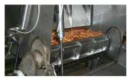
casings are removed and the product is ready to be fed to the packaging equipment. This manufacturer, like many others, used belt conveyors because they allowed for less upfront expenses over other conveying options. As this manufacturer found out, the skinless hotdogs were dragged along the interior walls' belt line seams. The fragile product can be easily deformed or broken at this stage in the process and that is where a horizontal motion accumulation conveyor
