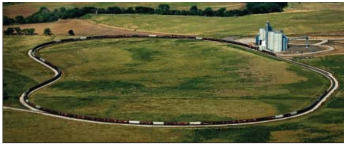
The shuttle terminal at Culbertson includes an 8,800-foot loop track. Photo by Lori Beguin.
