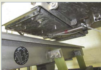
Original gate design required unbolting the gate plate to clean.
