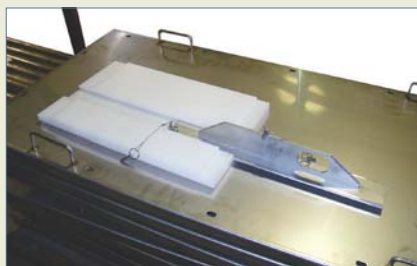
From underside of pan, UHMW gate slides onto mounting bracket.
