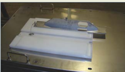
Gate plate with mounting bracket removed.
