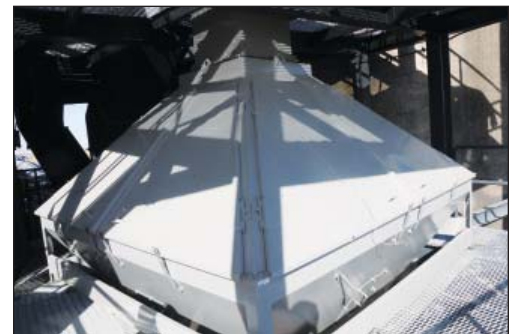
A new InterSystems gravity screener sits below the Texas Shaker.
