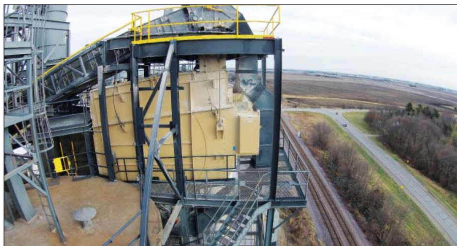
Aerial view of West Central's new Triple/S Dynamics Texas Shaker 60,000-bph grain cleaner in Boone, IA. Aerial photos by Adam Moeller, Moeller Engineering, Ankeny, IA.
