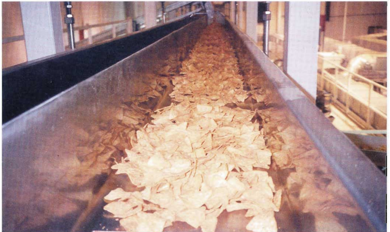
This horizontal-motion conveyor's gentle impelling motion enables it to transfer fragile tortilla chips without damaging them. The trough conveying section is stainless steel.
