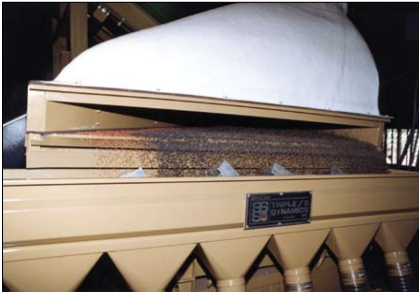
FIGURE 3. While the automation and control techniques for gravity separators are quite advanced, a typical modern gravity separator, as shown here, has utilized the same operating principles for nearly 100 years
