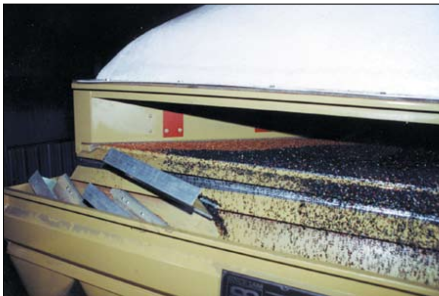
FIGURE 4. Processing a chopped power cable to recover its copper content is an example of a gravity separation where the "heavy" fraction (in this case, copper) must be isolated from the "light" fraction
