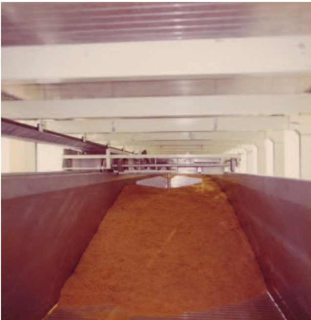
Belt storage unit accumulating pasta
