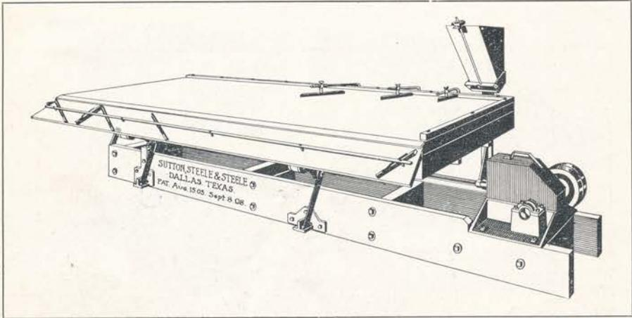
One of three valuable tables in our process with capacities from 10 to 15 tons on material all through 200 mesh, up to 200 tons on 4 mesh in 24 hours, and separates practically any free dry pulverant materials that have a difference in specific gravity of as much as one-half of one point.
