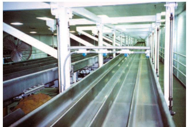
This horizontal-motion conveyor pan is fitted with multiple lanes that can singulate products during transport or transport different materials from multiple inlets to the same destination.
