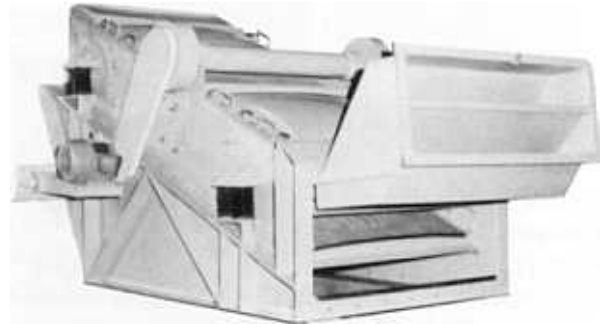
Stationary dust enclosure with hinged oversize chute in raised position for access to screen deck. Arrangement includes a base frame to level floor line with motor bracket. Sub-base bottom hopper for fines not shown.
