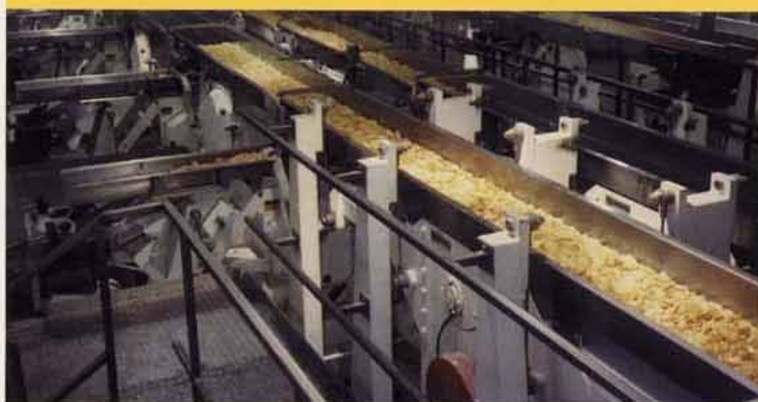
A Slipstick Modular Distribution System delivers product immediately on packaging demand.
