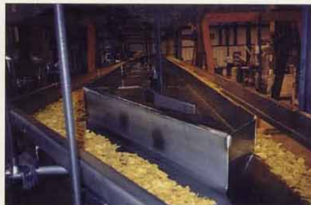
The use of product hold backs in the Slipstick system develops the surge or storage capacity of the conveyor pan.
