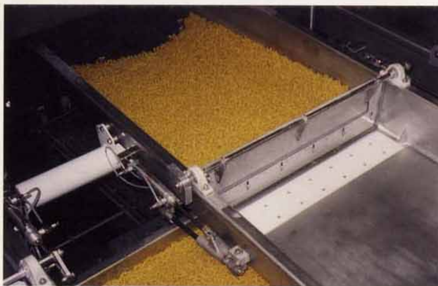
The use of product hold backs in the Slipstick system develops the surge or storage capacity of the conveyor pan.
