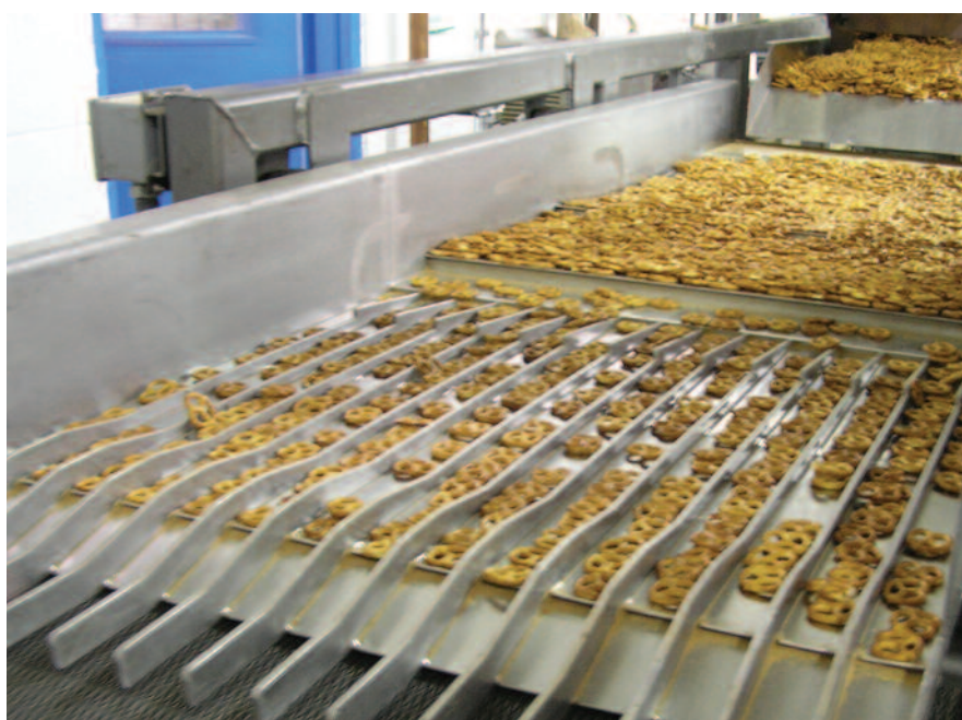
The conveyor trough's vertical lane-divider fins align the pretzels into single-file rows, which are transferred onto the enrobing line's belt conveyor.
